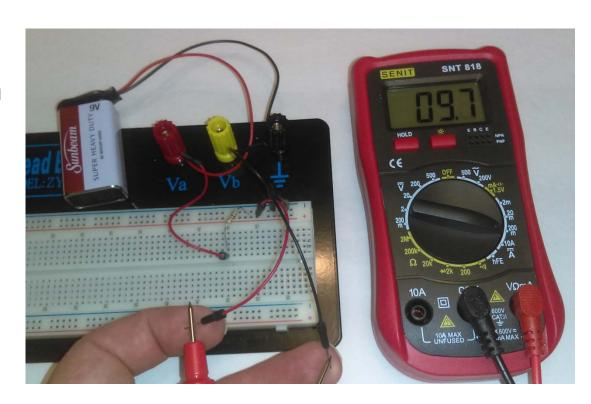
What is the best range to measure the current through a 1 k-ohm resistor?
