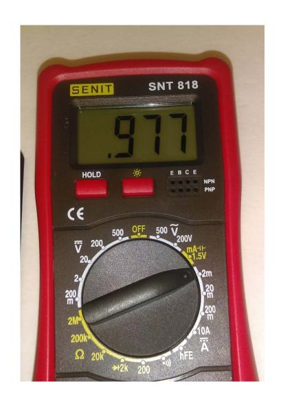
What is the best range to use to measure the current through a 10 k-ohm resistor at 9 volts?
